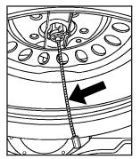
2. If the cable is visible, place the wrench on the hoist drive nut and turn the wrench counterclockwise until approximately 6 inches (15 cm) of cable is exposed.
